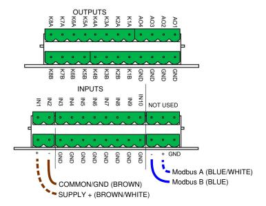
To power the expander from the ezeio, connect the the DC+ wire from the RJ45-jack to the + terminal on the expander as shown to the left.
